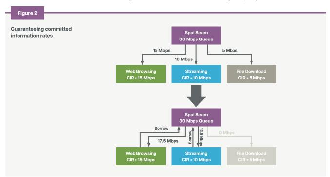
In **Figure 2** (above), bandwidth borrowing allows service providers to implement a series of hierarchical queues, where each child queue is guaranteed a committed information rate. Here the spot beam represents the parent queue, and the child queues represent sub-elements utilizing the beam, such as, an application group, an aircraft, a sea vessel, or end users.
